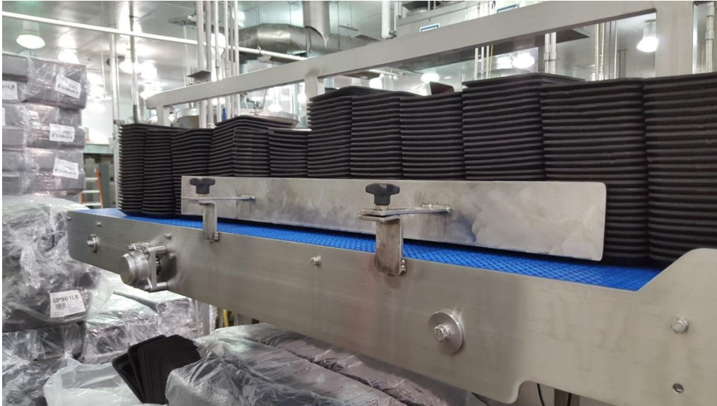
PREVIOUS TRAYS STACK ON THE PAD VERSUS THE SIDEWALLS LEADING TO UNSTABLE STACKS
