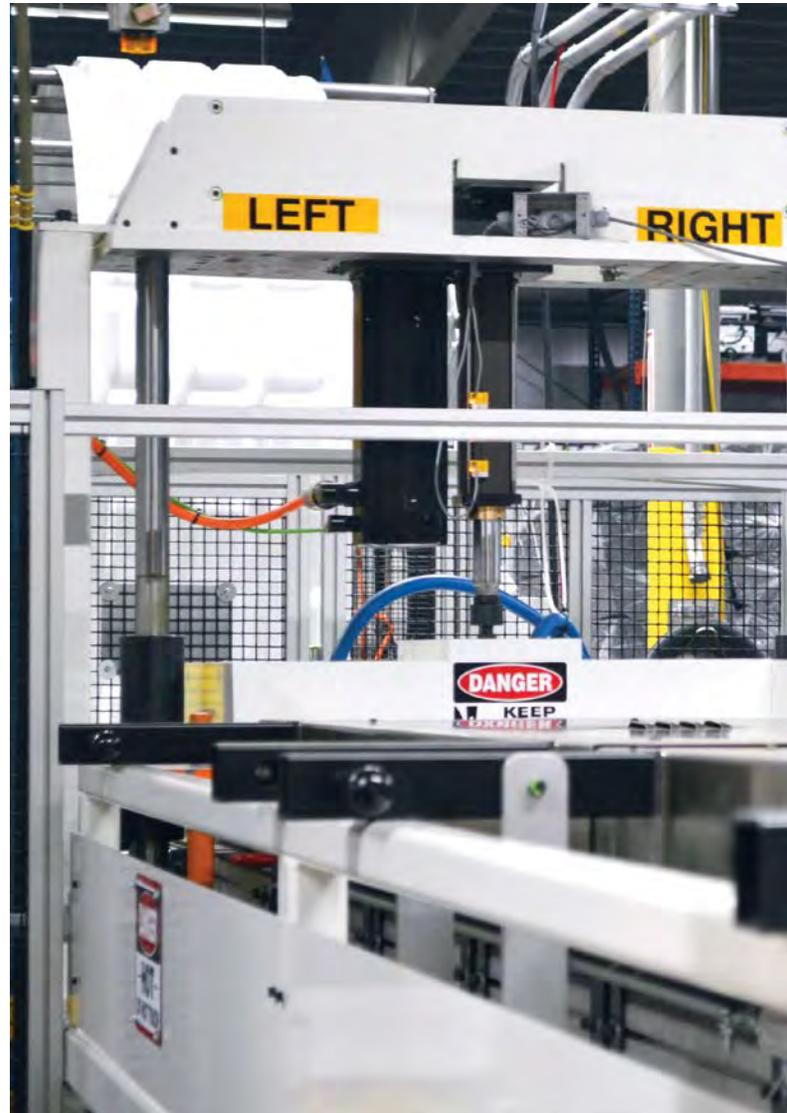
cycle. Furthermore, a power canopy is utilized to present the formed sheet to the trim tool feeder rather than attempting to pull the entire sheet from the form station over the canopy to the trim tool. Having an intermediate step to stage the sheet reduces tension on the material which improves trim accuracy.
